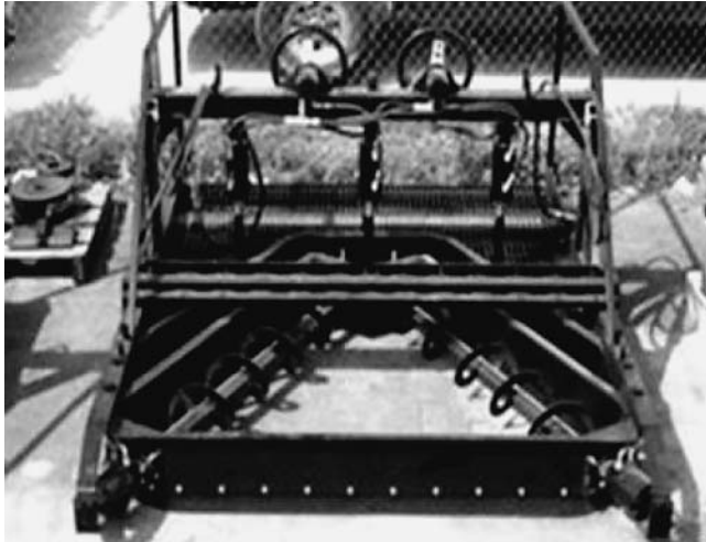
FIGURE 19 Rut box (Courtesy: Bergkamp Inc. 2010).
