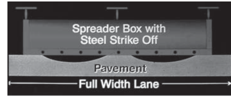
FIGURE 18 Scratch coat diagram (ISSA 2010a).
