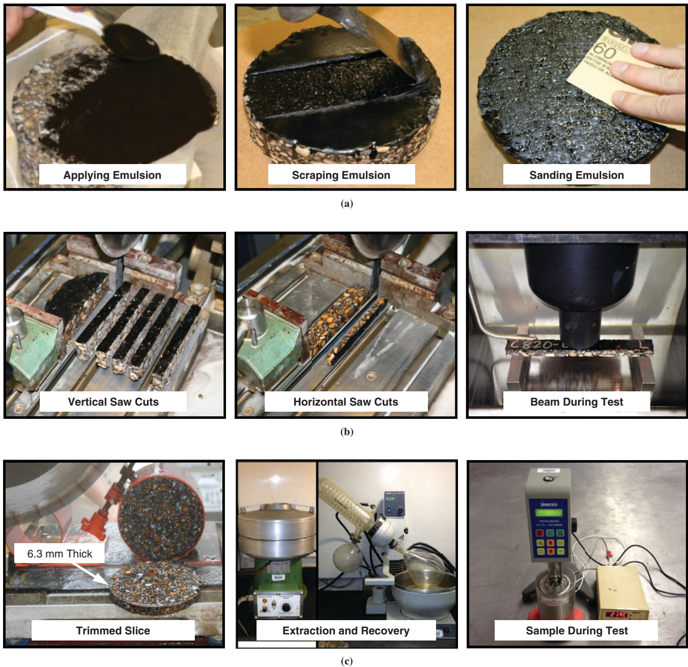
FIGURE 1 Specimen fabrication and testing procedures: (a) emulsion treatment procedures, (b) BBR beam sawing and testing, and (c) viscosity slicing and testing.
